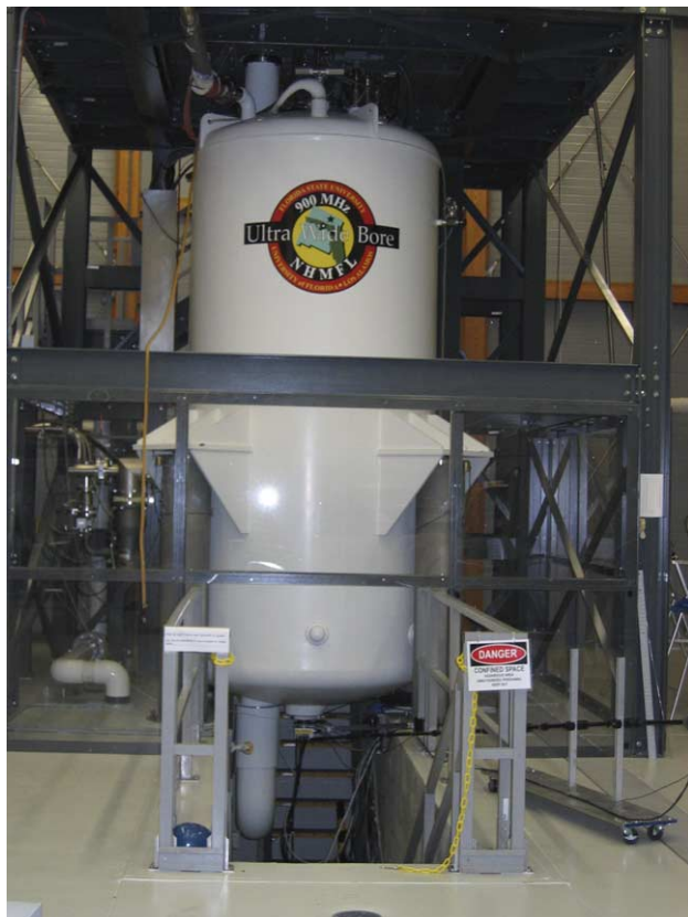
Fig. 1. Ultra wide bore 900 MHz NMR magnet system at the National High Magnetic Field Laboratory.
