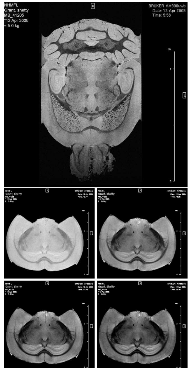
Fig. 6. Gradient-recall echo images of an excised, perfusion-fixed C57BL/6J mouse brain in a 10-mm linear birdcage recorded at 21.1 T. A true 3D gradient-recall echo dataset was acquired at a resolution of 18 \times 18 \times 35 \mu\text{m} in 29 h using the following imaging parameters: matrix = 1024 \times 512 \times 256 ; TE/TR = 12.5/100 ms; averages = 8; FOV = 1.9 \times 0.92 \times 0.8 cm; bandwidth = 100 kHz; 50^\circ tip angle = 25- \mu\text{s} hard pulse. A series of 2D multi-slice gradient-recall echo images ( 40 \times 40 \times 250 - \mu\text{m} resolution) were acquired to sample T_2^* using the following parameters: matrix = 230 \times 200 ; TE = 4.5–24.5 ms; TR = 1.5 s; averages = 2; FOV = 9.2 \times 8.0 mm; slice thickness = 250 \mu\text{m} ; number of slices = 17; 90^\circ pulse = 2-ms three-lobe sinc pulse; and imaging time per dataset = 10 min.
